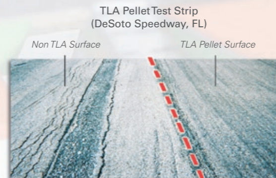
Comparison of TLA Pellets vs. Non TLA Surface after 4 years.
